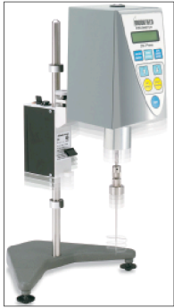
Figure 1: Brookfield Viscometer with T-Bar Spindle for Testing Peanut Butter and Yogurt
